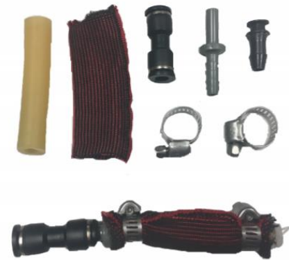
Figure 10. Hydromuscle Materials and Construction (Curran et al., 2018)
