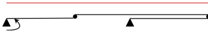
Figure 3.2: Singular position of parallel 4-bar linkage, in which all links overlap into one single line
