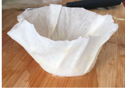
Figure 2: A paper towel soaked in adhesive molded around a cup
