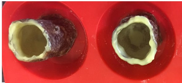
Figure 50: Candelilla Wax Coated Cups Filled with Water for 24 Hours
