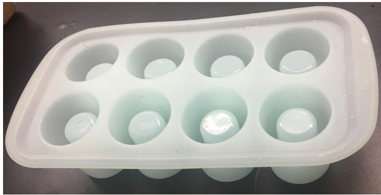
Figure 34: Silicone Mold for Cylindrical Cups
