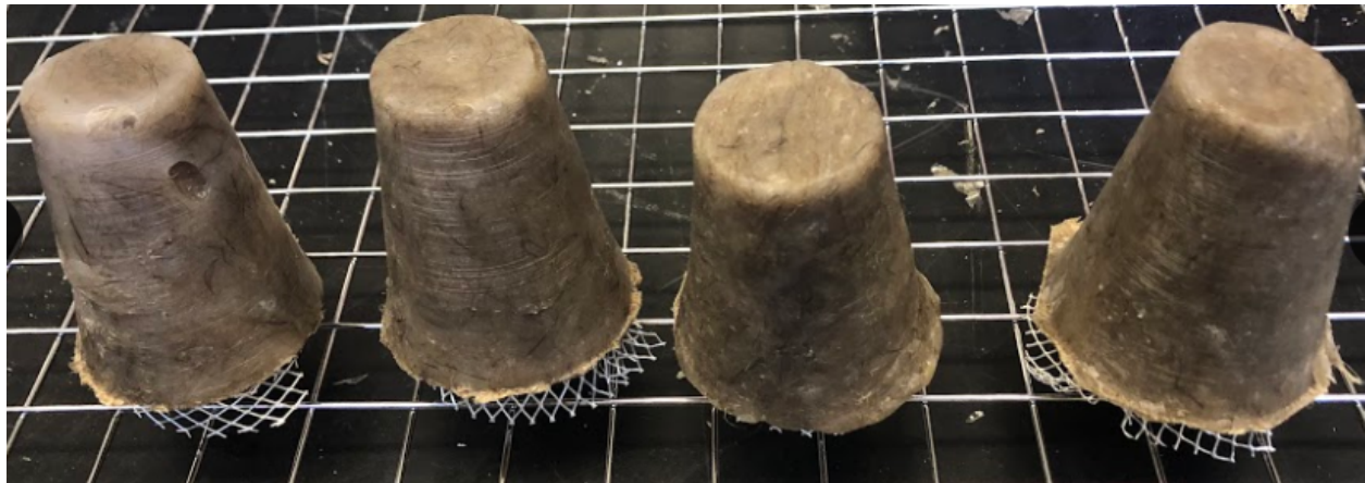
Figure 8: Cooled Hemp-Agar Pulp on Mesh Drying Mold
