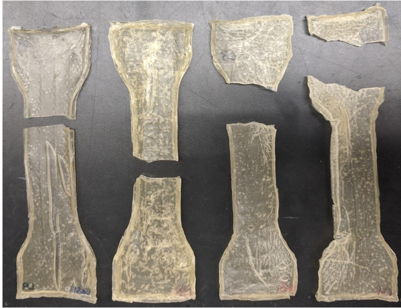
Figure 20: Post-testing Cornstarch Samples
