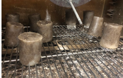
Figure 9: Hemp-Agar Cup Samples in Convection Oven.
