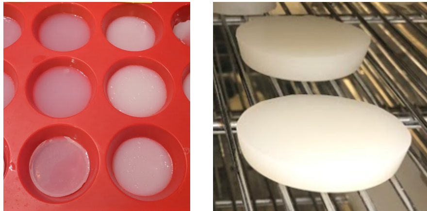
Figure 23: Puck Mold and Wet Pucks in Oven for Mold Testing
