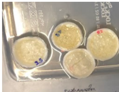
Figure 38: Half-submerged Pucks in Hot Water at End of Testing
