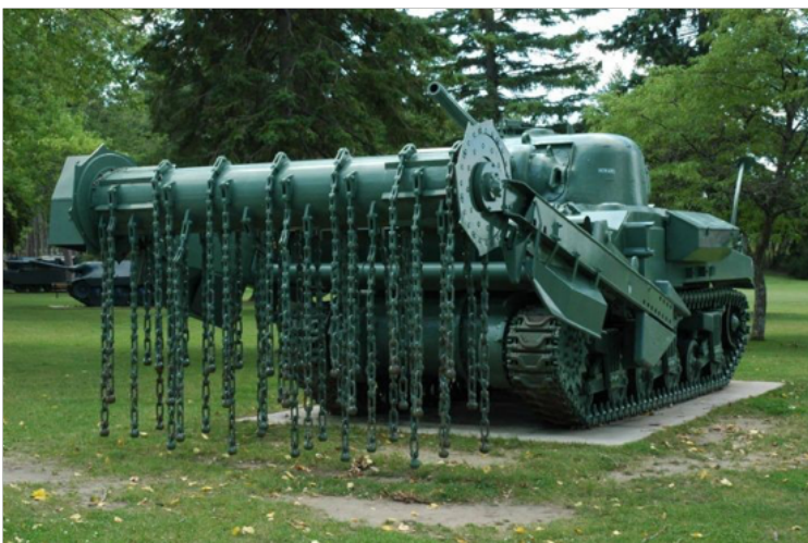
Figure 2.7: Image of landmine flail tank (GRB 1 933, 2010)
