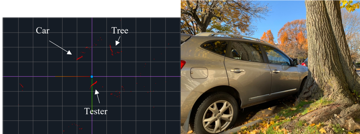
Figure 12: LIDAR point cloud and actual objects
