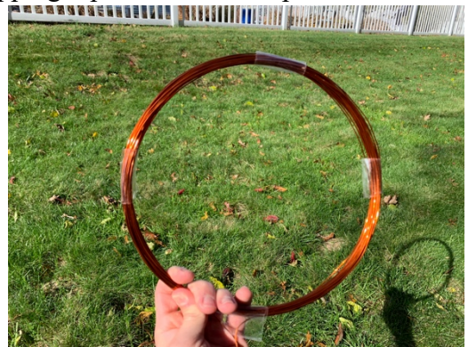
Figure 1: Coil Winding and tape placement
