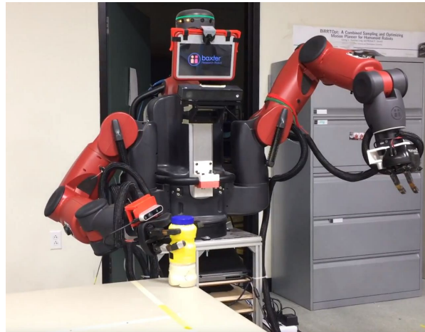
Figure 24: The Kinect is mounted on the Baxter's upper 'chest'.
