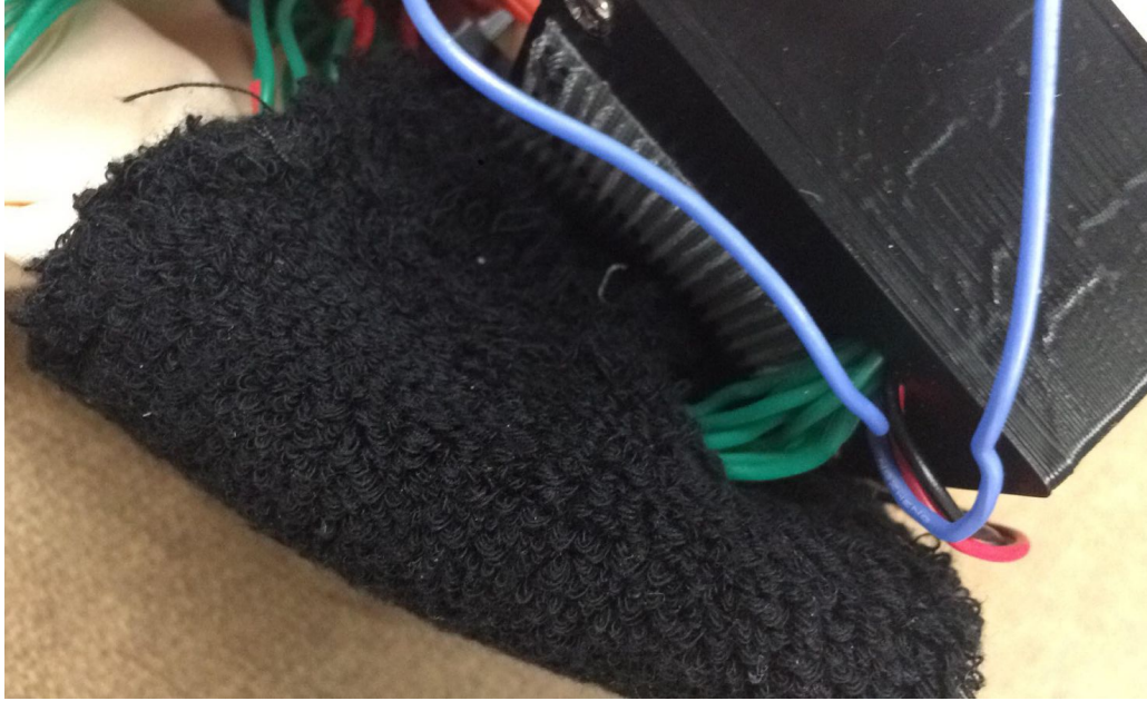
Figure 17: Wiring of the PCB to the Glove
