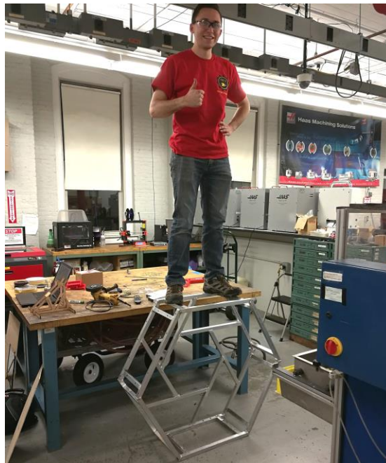
Figure 12: Aluminum Frame Supporting ~170lbs
