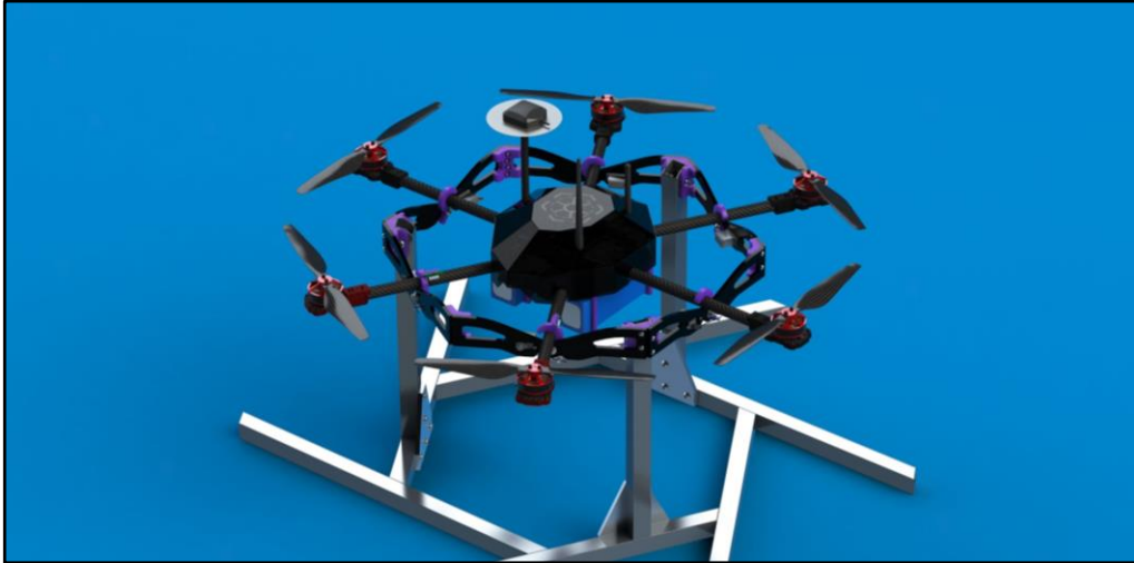
Figure 14: Render of Base Station Landing Ring
