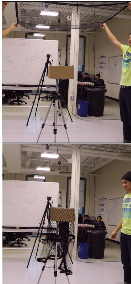
Figure 16. Physical net drop using Vicon cameras
