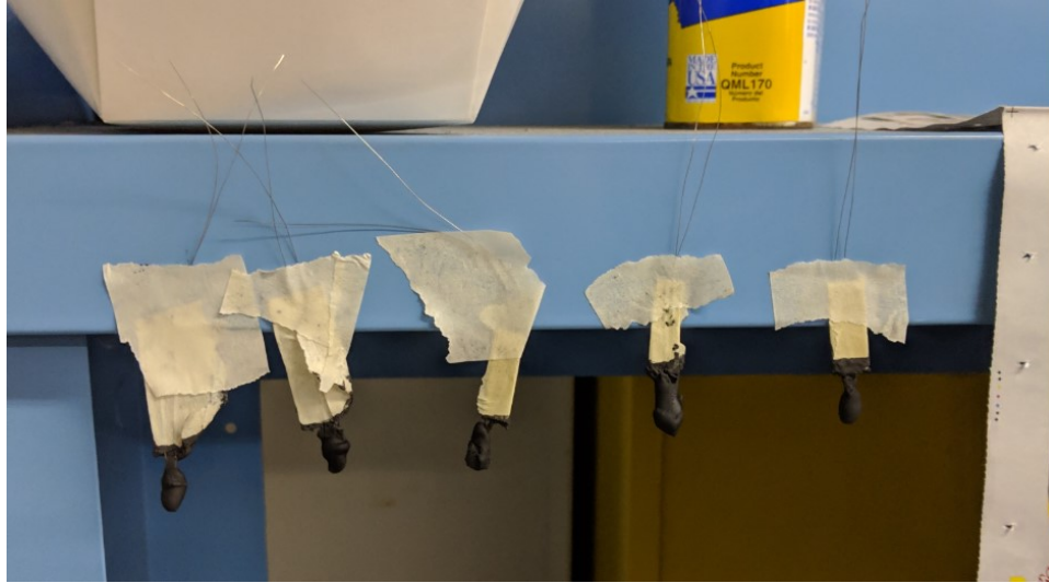
Figure 2.8. First attempt constructing electric match ignitors. Ignitors are shown taped to workbench to allow drying.
