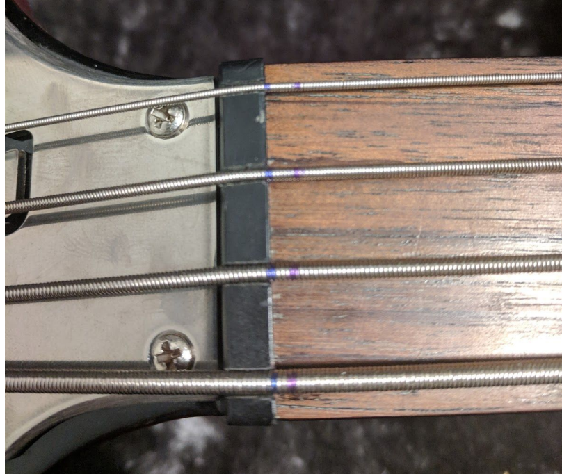
Figure 6: The test bass, with string markings for highest and lowest tensions. Bass is shown with strings at lowest tension.
