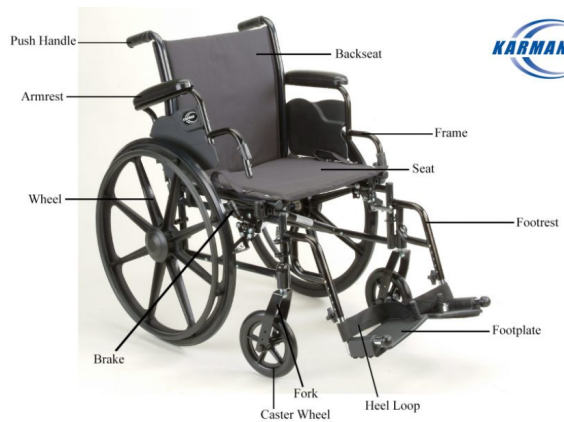
Figure 3: Manual Wheelchair Components [11]
