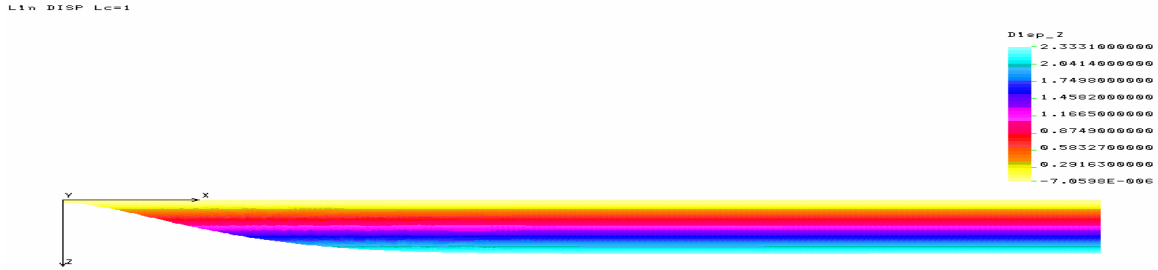
Fig. 7.15. Deformation of the diaphragm in z -direction.
