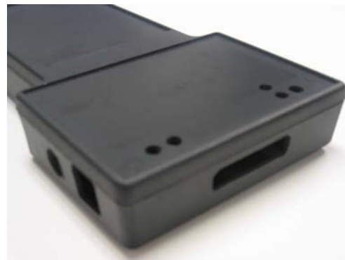
Figure 77: Closeup of Enclosure Cutouts
