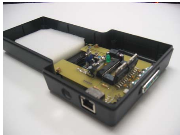
Figure 82: PCB Mounted Within Enclosure
