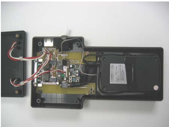
Figure 84: Battery and Power Switch Installed
