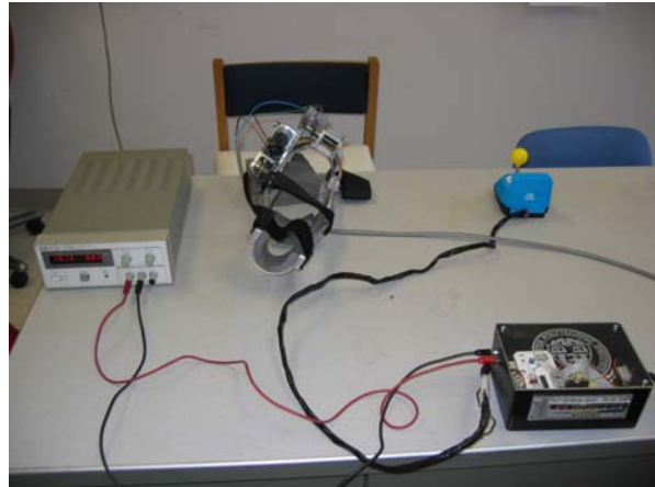
Figure 19: Prototype with power source, and control system
