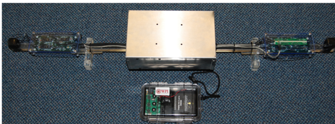
Figure 1.4: Mantenna Version 4 Receiver Wand and Transmitter
