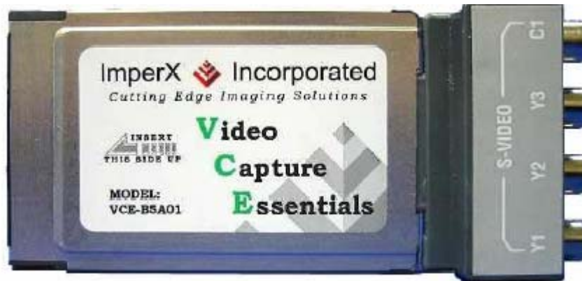
Figure 3-15: PCMCIA frame grabber (courtesy Imperx)
