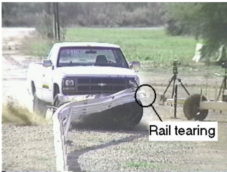
Figure 51: Crash sequence at rail rupture (TTI 473750-1).
