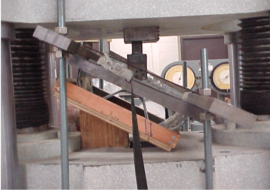
Figure 38: Test setup for the 30/0 degree load test.
