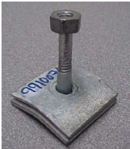
Figure 42: The result of test 99100701 showing the failed components.
