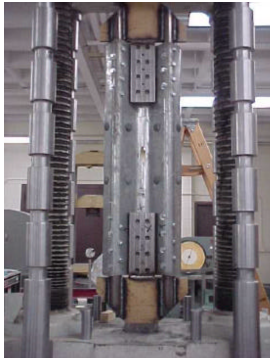
Figure 8: Uniaxial tensile test setup.
