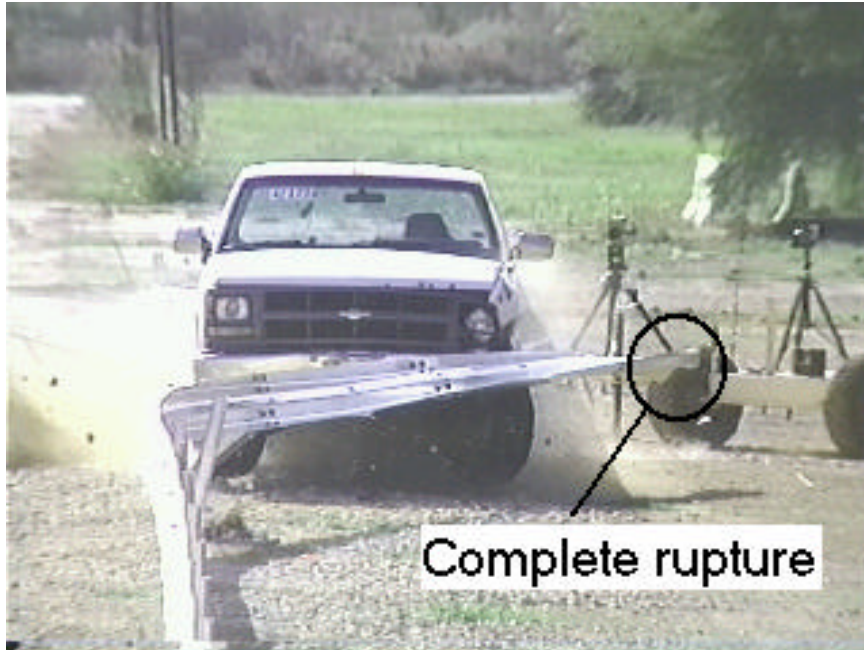
Figure 52: Crash sequence after rail rupture (TTI 473750-1).
