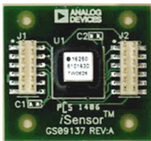
Figure 3.4: Analog Devices ADIS16255 single-axis MEMS CVG evaluation module [6]
