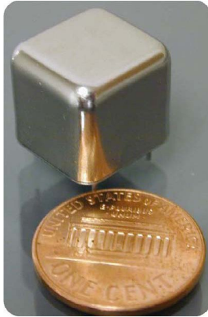
Figure 3.3: Gyration MG1101a dual-axis MEMS CVG [5]
