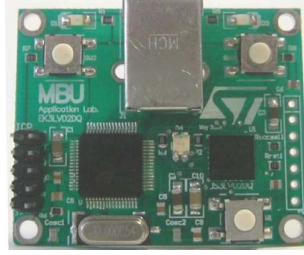
Figure 3.9: LIS3LV02DL Tri-Axis linear accelerometer evaluation module
