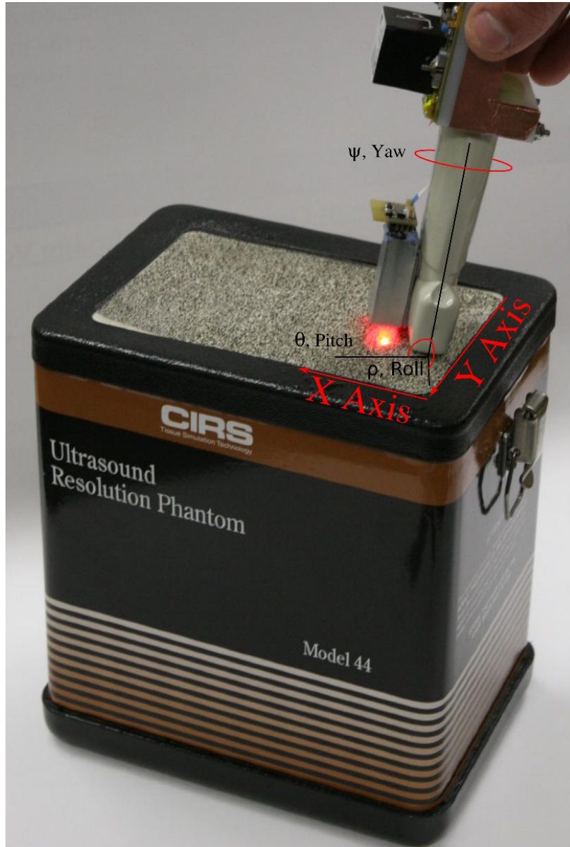
Figure 10.1: Reference coordinate system relative to the ultrasound phantom. The x and y axes illustrated here correspond with those used throughout the testing.
