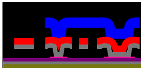
Fig. 2.6. 2D representation of the cross section of the anchor hinge along line A-A (Pryputniewicz and Furlong, 2003).
