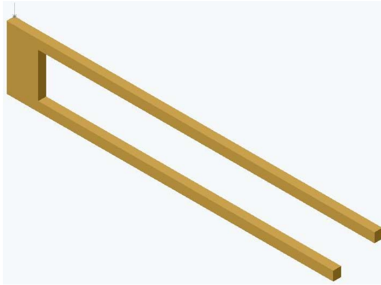
Fig. 4.9. SolidWorks representation of the folded spring used in the Sandia microgyro.
