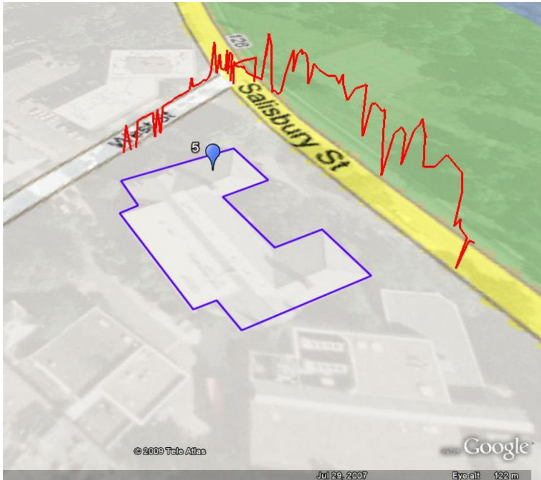
Figure 3-8 RSS signature of AP 5 in AK plotted on Google Map showing the location and length relative to the location of the AP in the building
