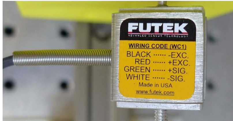
Figure 2.7: The load cell connected to the amplifier
