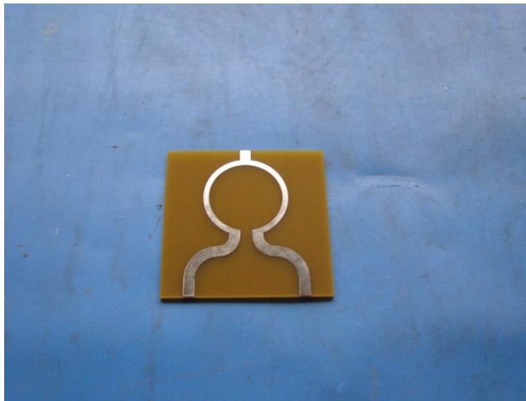
Fig. 30: 2:1 power divider, without connectors and chip resistors soldered.
