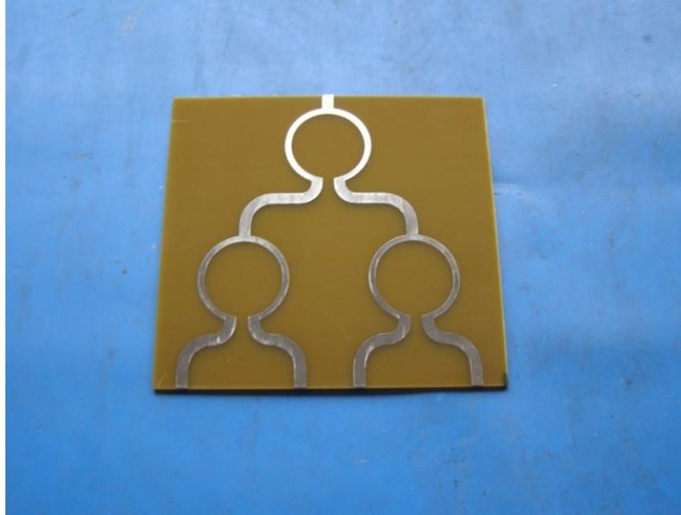
Fig. 31: 4:1 power divider, without connectors and chip resistors soldered.
