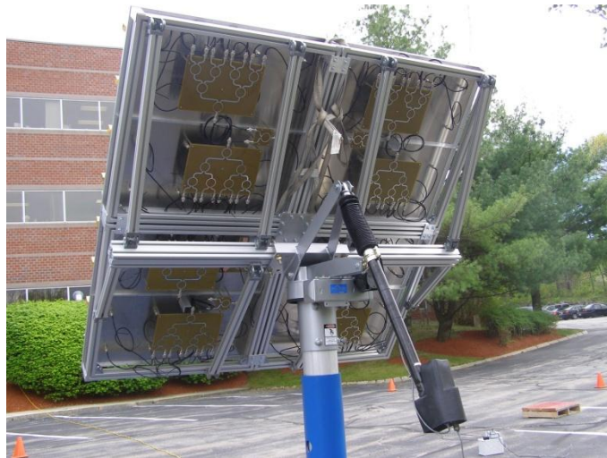
Fig. 47: Array assembly. Back view with the feeding network (Courtesy of Physical Sciences Inc.).
