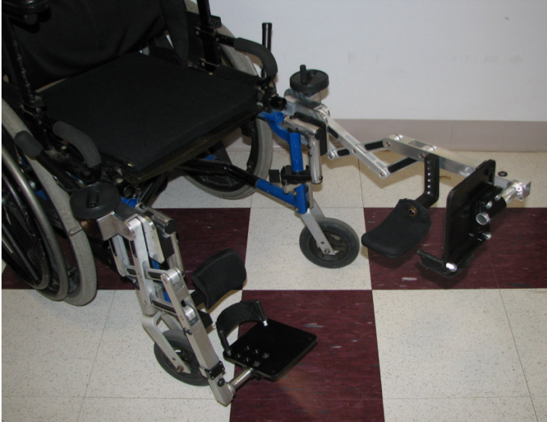
Figure 58: Quickie wheelchair with legrest prototypes attached - one lowered, one elevated
