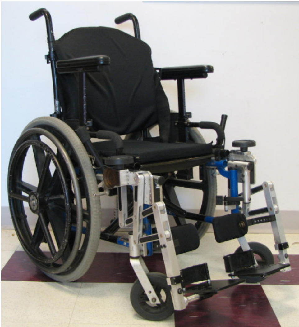
Figure 57: Standard Quickie wheelchair with legrest prototypes attached in the lowered position
