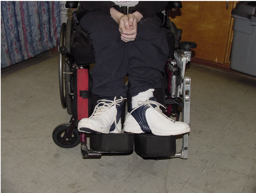
Figure 61: Test client Andy with original elevating legrest on his right and the adjusted legrest prototype on his left (including footrest blocking, larger calf pad, and pull-to-lock wheel lock)
