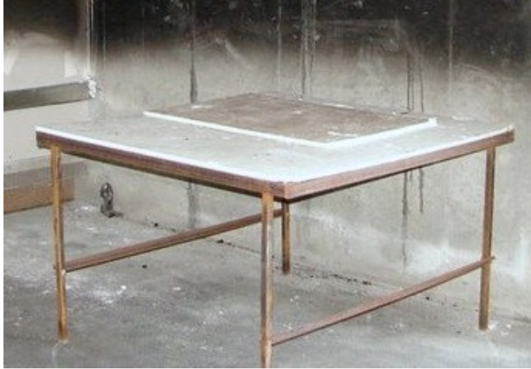
Figure 4-18: Non-combustible "prop" table
