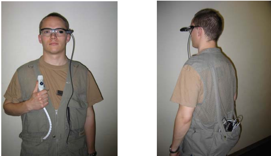
Figure 9.1: Second generation ultrasound scanner system
