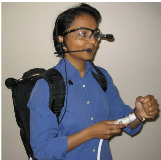
Figure 3.2: Photograph of a person wearing the ultrasound scanner system
