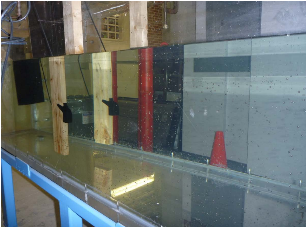
Figure 18: Two transducers oriented towards the same wall to measure the reflected signal.
