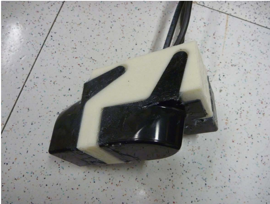
Figure 36: Completely assembled sensor housing for the sonar module.
