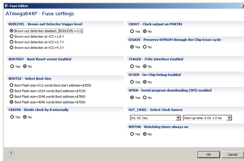
Figure C.5: Worksheet for setting internal fuses.
