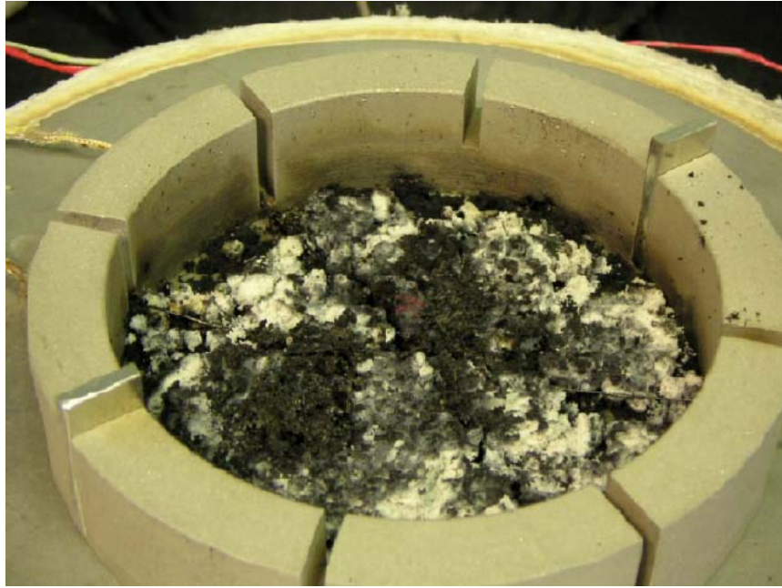
Figure 57 : Gum powder (20g) with ketone-based liquid solution (2g), at the end of test
