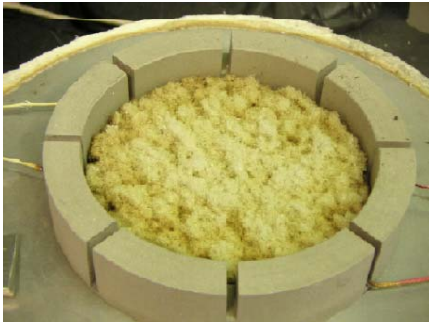
Figure 22 : Paper dust layer right after being leveled at 350\text{ }^{\circ}\text{C}
