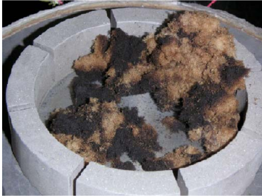
Figure 24 : Chars formed on the bottom of paper dust layer at 350°C
