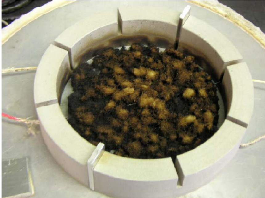
Figure 38 : Paper dust (3g) with DTE24 (3g) at 400°C, at the end of test
