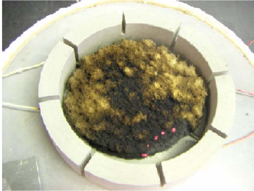
Figure 26 : Glowing in the paper dust layer at 360°C
