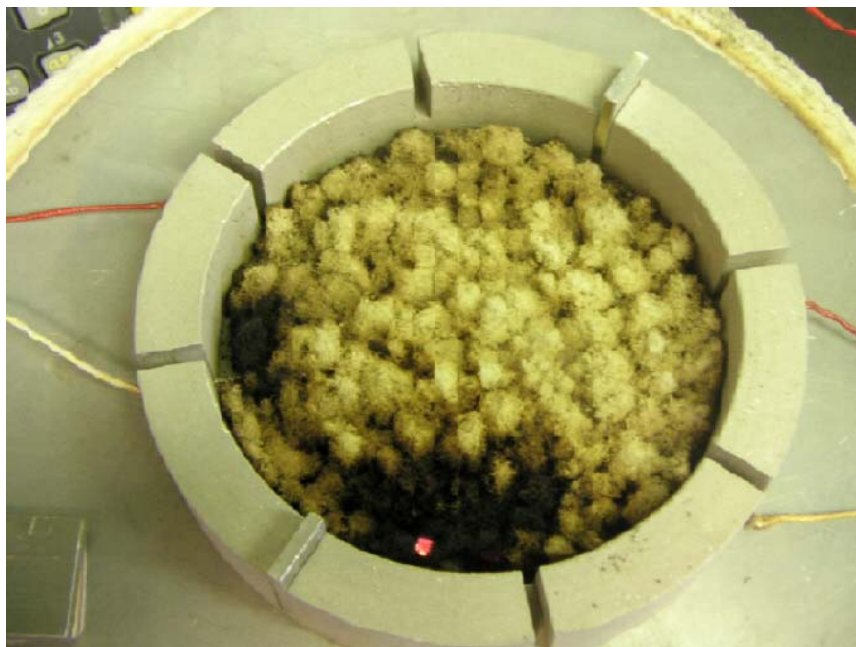
Figure 46 : Paper dust (3g) with n-decane (3g) at 360°C
