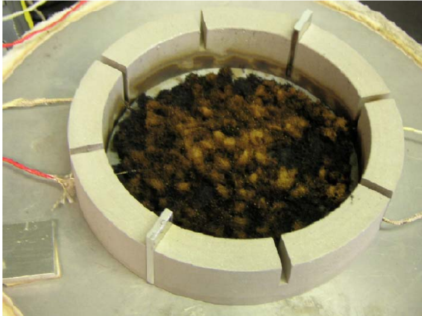
Figure 35 : Paper dust (3g) with Citgo oil (3g) at 400 °C, at the end of test
