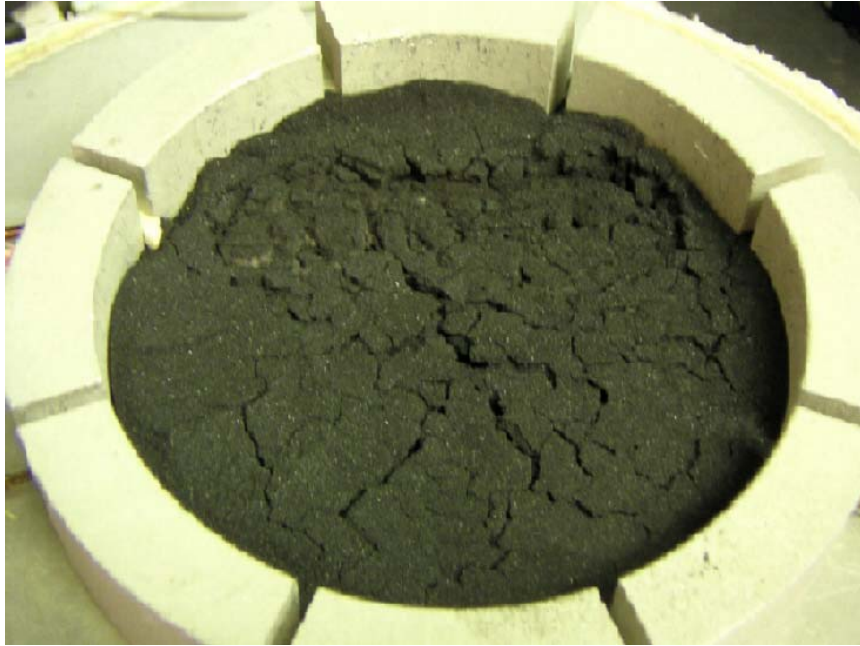
Figure 74 : Pittsburgh seam coal when ignition occurred
