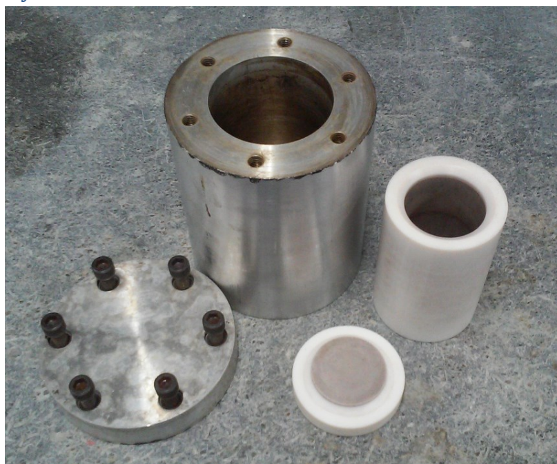
Figure 54. Autoclave (left) and teflon liner (right). The caps are shown next to the container. The Teflon liner cap is held in place by the autoclave cap, which is screwed in place using a hex key.
