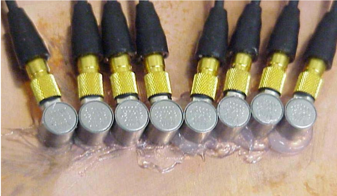
Figure 6-4: Eight transducers mounted to the copper block. In this experimental setup, the eight transducers were placed in a linear array as closely spaced as possible for maximum spatial resolution. Each transducer is \frac{1}{2} " in diameter.
