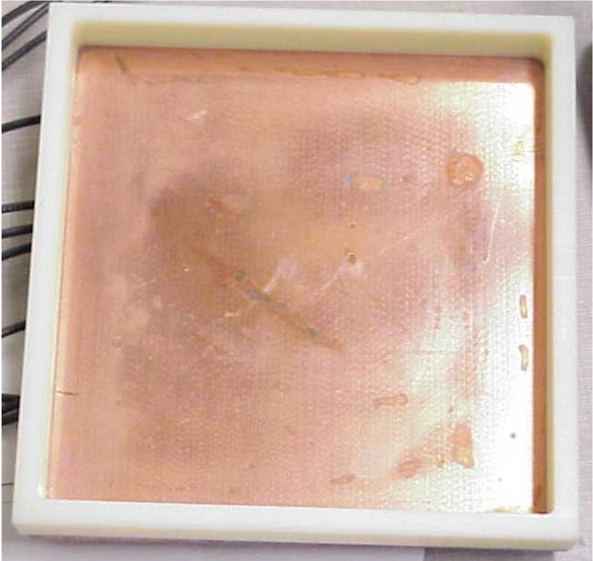
Figure 6-8: Second experimental test block with polyethylene rim. Unlike the first block, this was simply a solid block of copper with no cooling channels.
