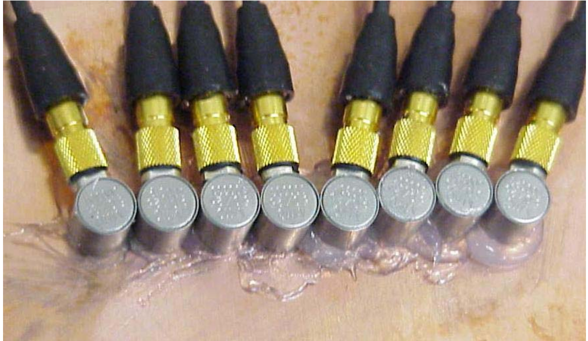
Figure A-4: A close-up view of the mounted transducers; excess silicone sealant was wiped away before it dried.
