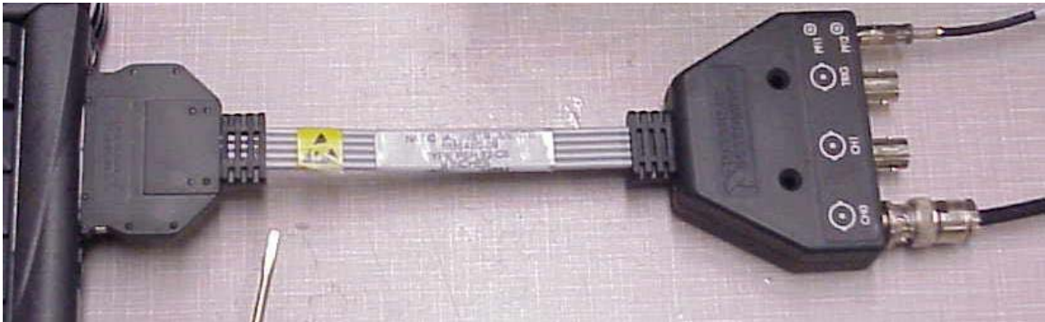
Figure 6-2: Digitizer card connector cable. The card itself is in the computer's expansion bay at the left of the photo, with the cable plugged into it. At the right of the photo is the terminal block holding all of the connectors which lead to the digitizer.
