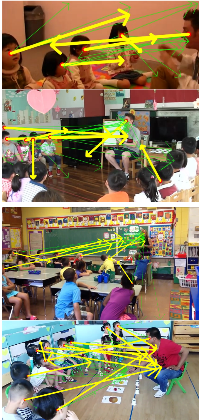
Figure 6.1: Handpicked qualitative results of gaze predictions by Merged Model using regression approach on test set. Thin green arrows are ground truth annotations. Since there are multiple gaze annotations for each individual, there are multiple green arrows for each individual. Thick yellow arrows are predictions by Merged Model. Images (top to bottom) taken from: https://goo.gl/xUdYbC , https://goo.gl/FBSA57 , https://goo.gl/v931J6 , https://goo.gl/pcwQ5P
