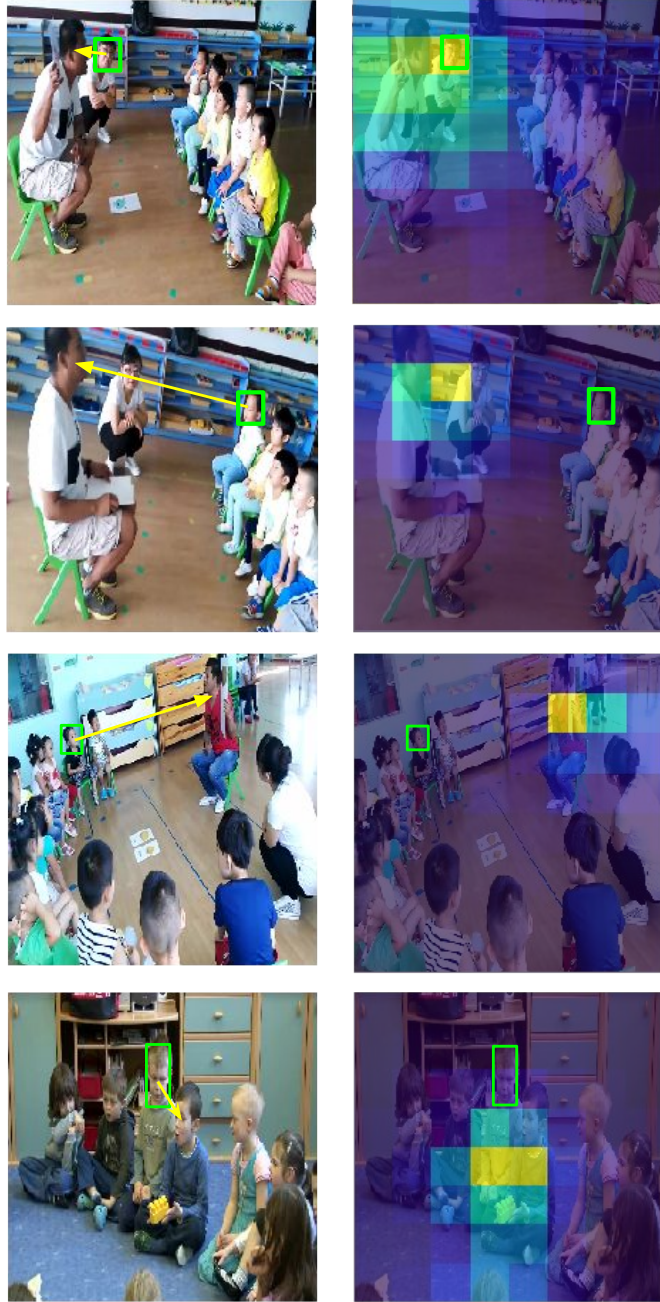
Figure 6.2: Handpicked qualitative results of gaze prediction by Merged Model using classification approach on test set. Left Column: Input images resized to 256 \times 256 pixels. Green bounding boxes are person of whose gaze are being predicted and yellow lines are human labeled gaze annotations. Right Column: Softmax output distribution on 8 \times 8 grid predicted by Merged Model for corresponding images and person of interest (indicated by green bounding box). Softmax output distribution forms a heatmap of the region of gaze by the person in green bounding box.
