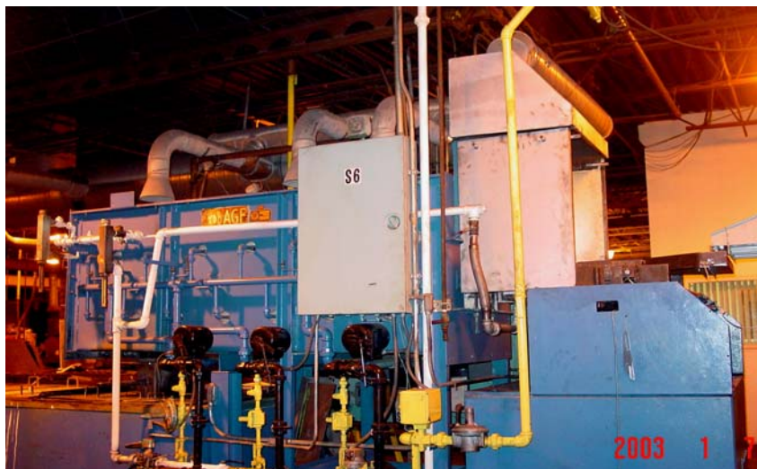
Fig. 58 Shaker Furnace used for the Case Study
