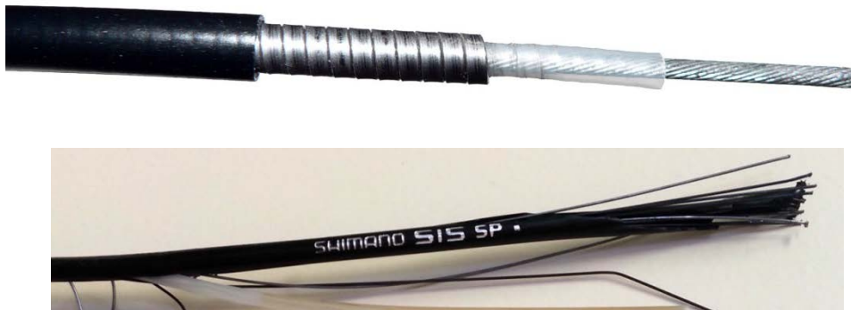
Figure 40 Bicycle break and shifter Bowden cables (31)
