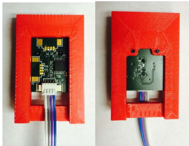
Figure 59 Magnetic Sensor Board Ready to be calibrated on the Manual Mill
