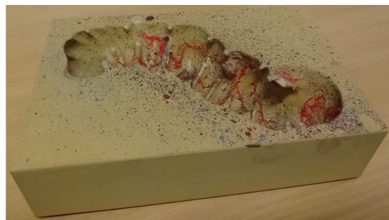
(b) A colon phantom is painted after 3D-printing in order to mimic the visual features of colonic mucosa
