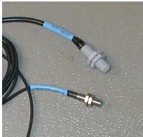
Figure 5.3 The two proximity sensors used for the case studies
