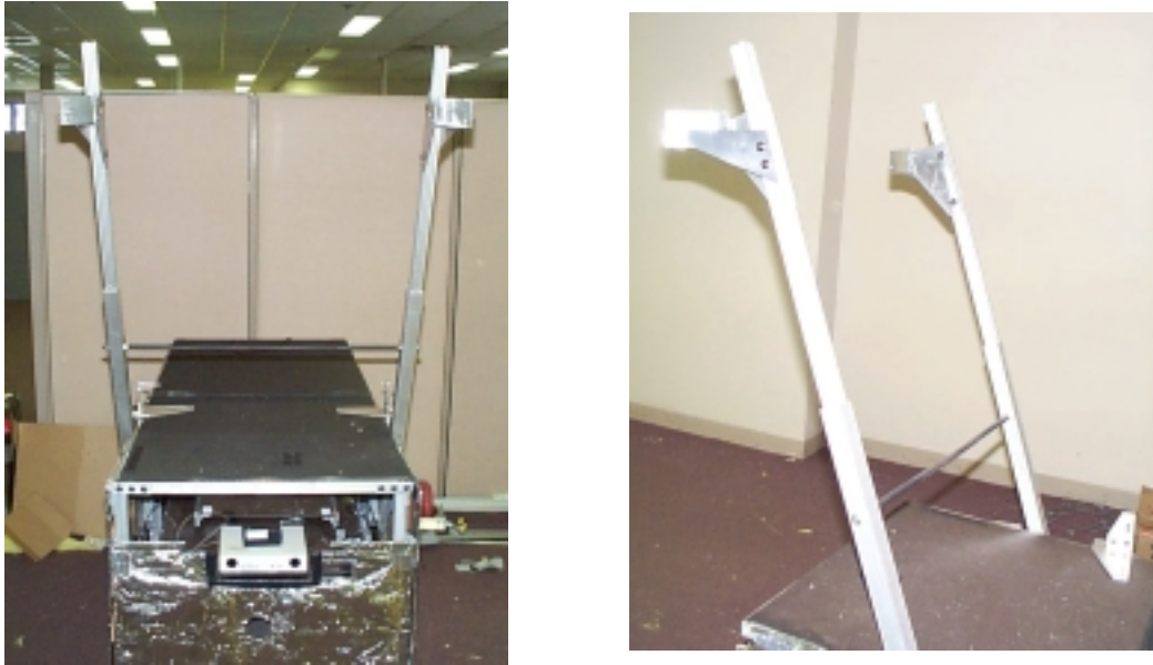
Figure A2.5: Front and side views of PLSS supports for EV crewmember donning/doffing
