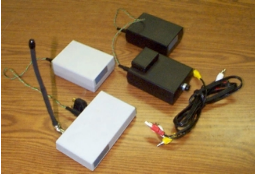
Figure 2.3: Pragmatic Communications Systems True View color camera, 900 MHz transmitter and receiver, and RCA cables
