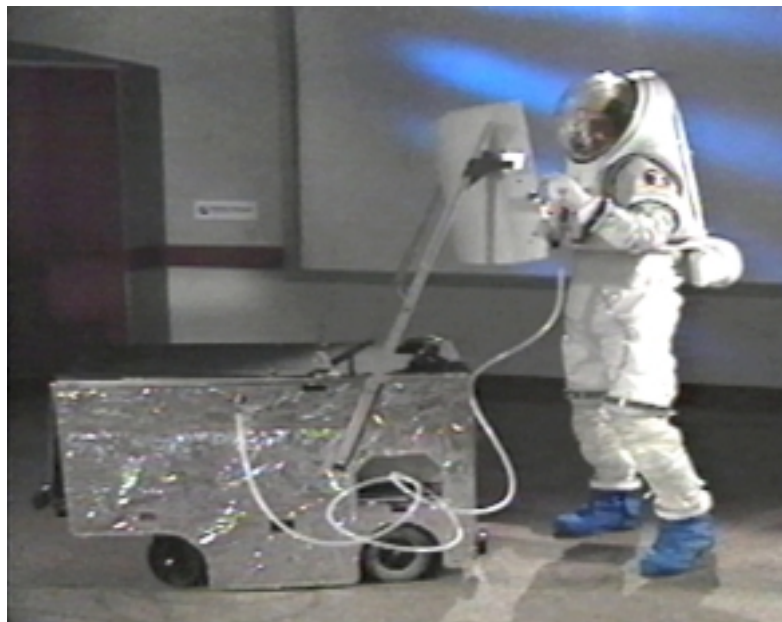
Figure A2.4: EV crewmember interfacing with FIDOE's on-board LSS via the O 2 port
