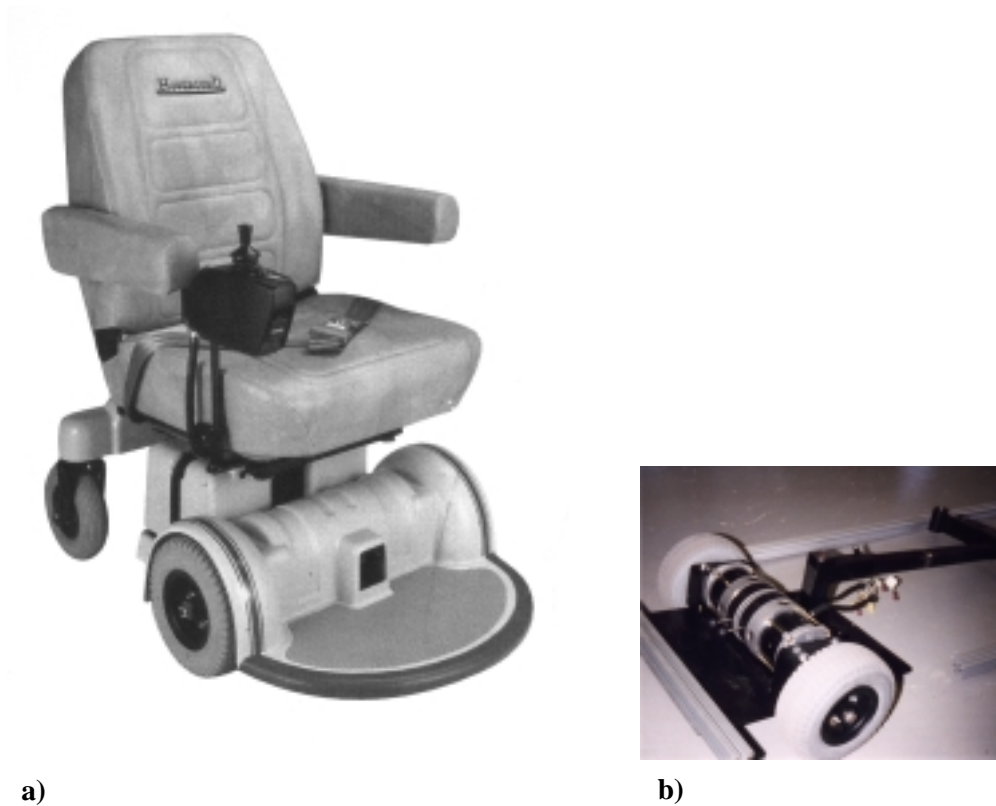
Figure 2.12: a) HoverRound MPV4 motorized wheelchair, b) Stripped-down motorized wheelchair with chassis modification
