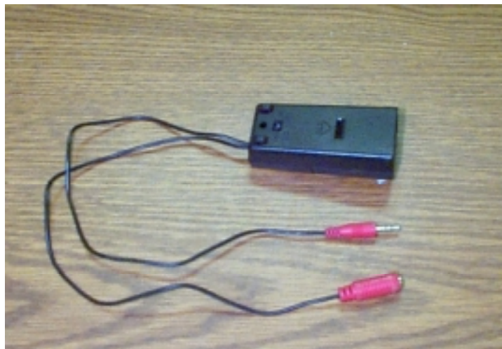
Figure 2.10: Dragon Dictate signal amplifier
