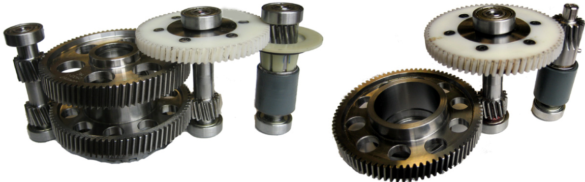
Figure 37 - Original Gear Train (Left) vs. Modified Gear Train (Right)
