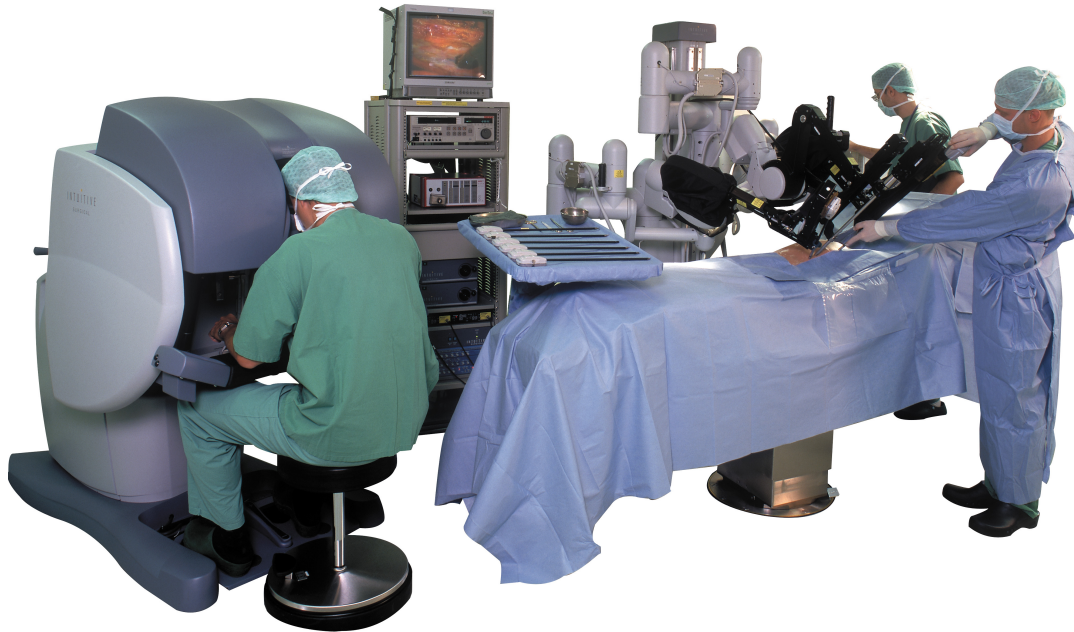
Figure 1.4: The daVinci Surgical System with the surgeon operating the MTM console and the helping nurse at the PSM station
