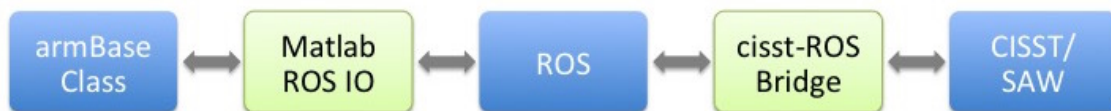
Figure 7.5: the armBase class connect to ROS using Matlab-ROS IO bridge and ROS connect to CISST/SAW using cisst-ROS Bridge. Thus there are two bridges in between to connect matlab code to dVRK manipulators
