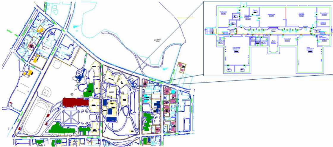
Figure 32: Merging the Kaven Hall floor plans with the campus map in AutoCAD
