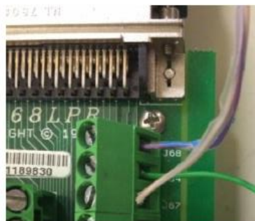
Figure 5: AMPL CMN and AMPL OUTPUT connected to J68 and J67 respectively. The green wire connected is unrelated to the load cell output.
