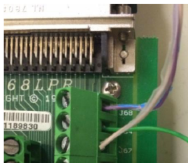
Figure 4: AMPL CMN and AMPL OUTPUT connected to J68 and J67 respectively. The green wire connected is unrelated to the load cell output.
