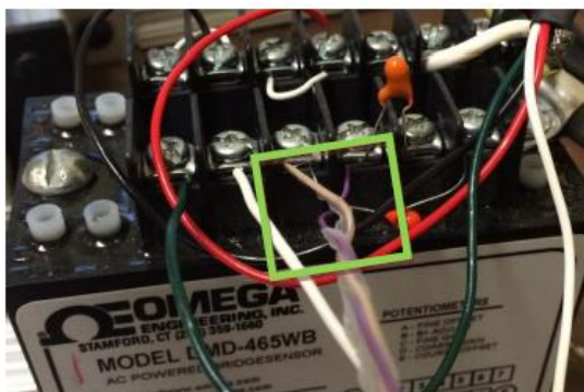
Figure 4: Side view of DMD-465WB with all connections. The amplifier output and common connections are located centrally in beige and purple.
