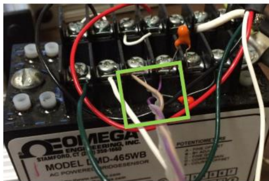
Figure 3: Side view of DMD-465WB with all connections. The amplifier output and common connections are located centrally in beige and purple.
