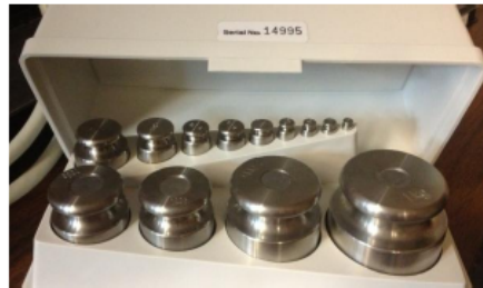
Figure 5: Calibrated mass set.
