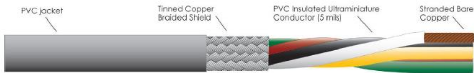
Fig. 2: Ultra-flex cable configuration
