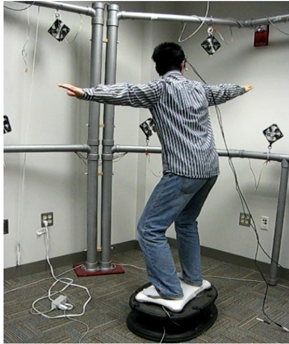
Figure 4.3: The TactaCage wind simulation system
