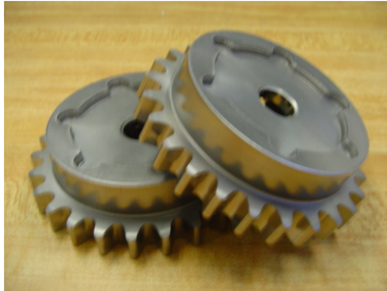
Figure 4.14: Green-state multilevel samples [33].
