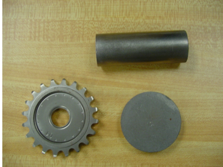
Figure 1.4: Various P/M parts: complex multi-level gear and uniform density cylinders.
