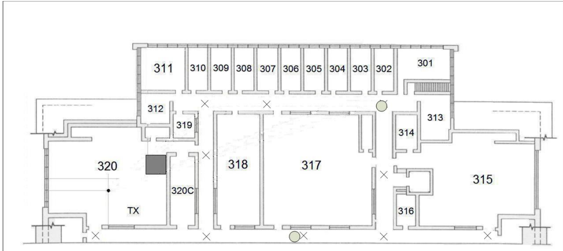
Figure 29: location of access points and training points for case II of scenario II
