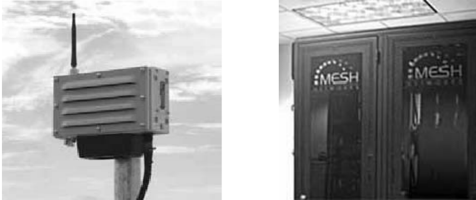
Figure 2.9: (a) Intelligent Access Points, (b) Mobile Internet Switching Controller (MiSC) in MEA.
