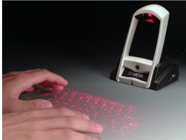
Figure 2.3: The Canesta keyboard uses hand recognition to allow for typing on any surface [13]
