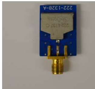
(c) Patch Antenna Working at 4.5 GHz
