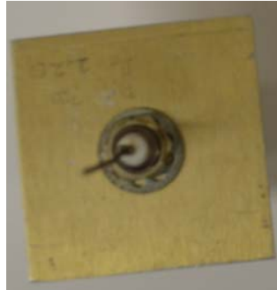
(b) Monopole Antenna Working at 2.25 GHz
