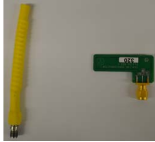
(a) Loop Antenna and Helical Antenna Working at 400 MHz
