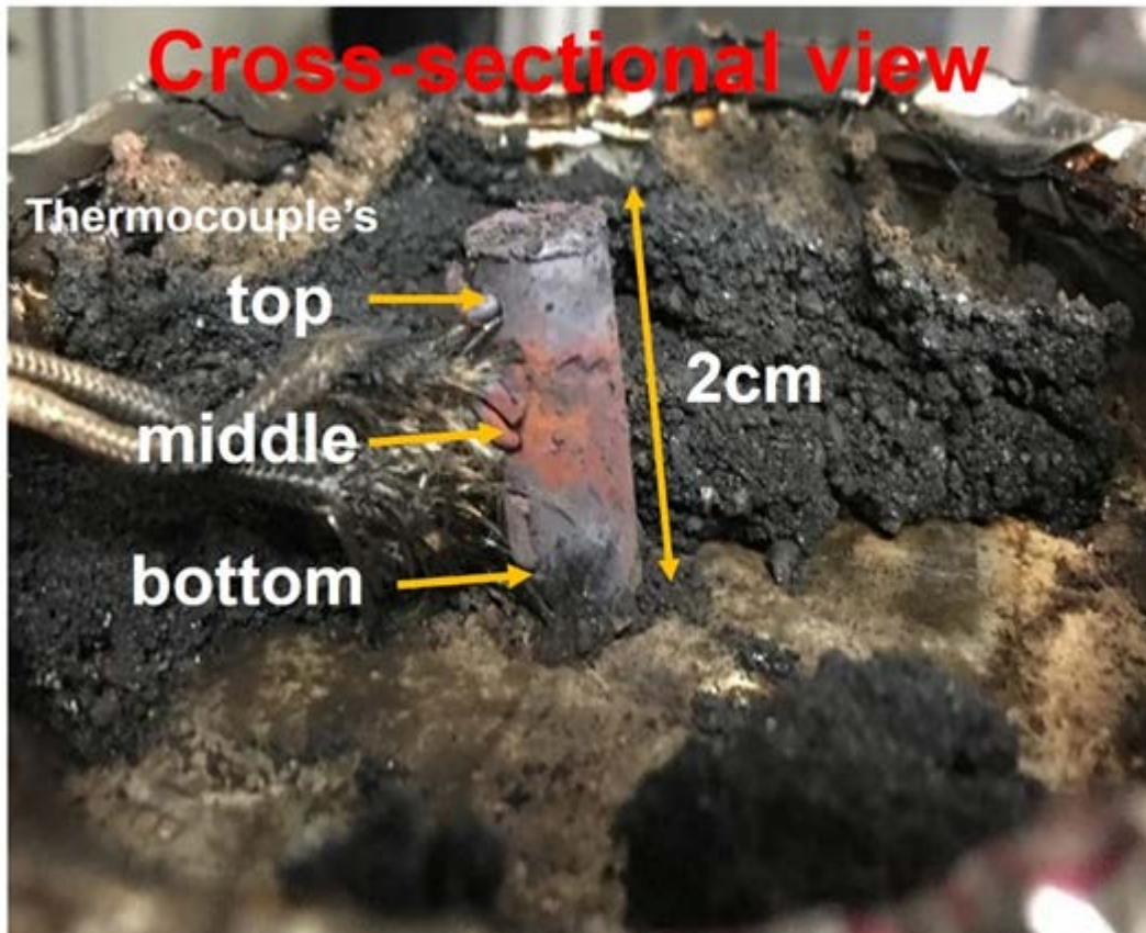
Figure 20: Cross-sectional view of burnt fuel at 25 kW/m 2 heat flux
