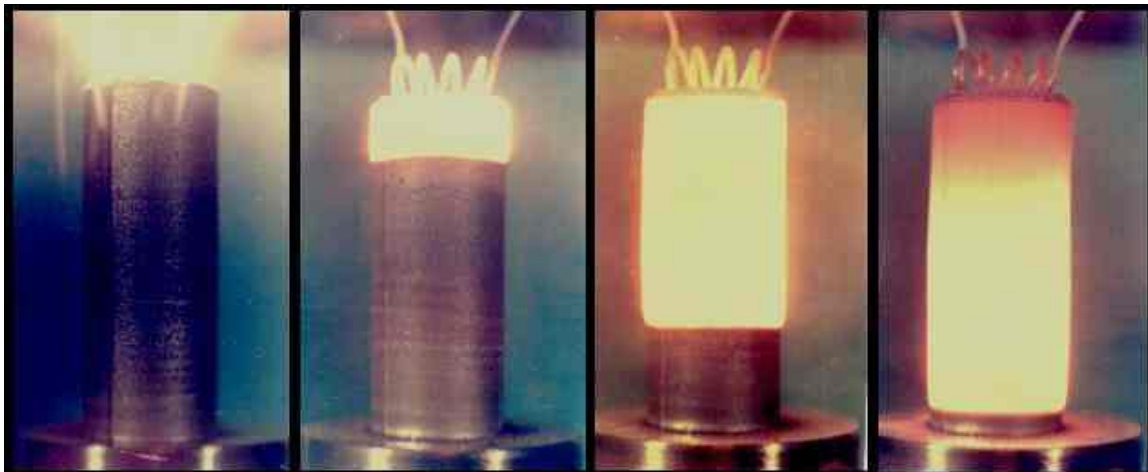
Figure 13: Combustion synthesis process
