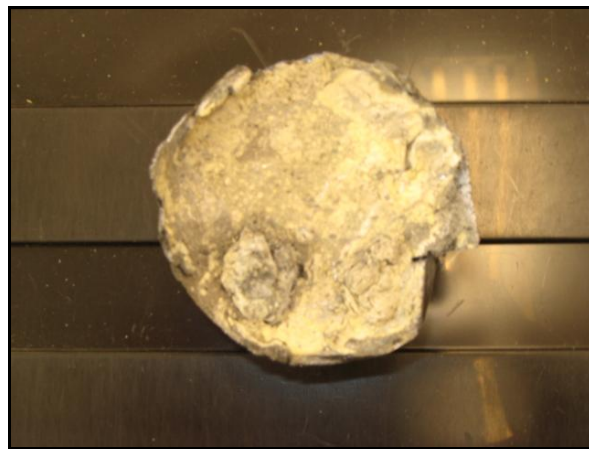
Figure 17: Yellowish layer of magnesium nitrides on the surface of the casting
