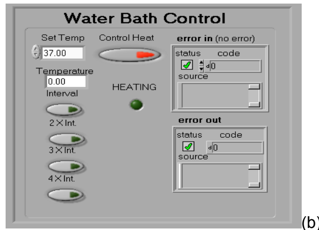
Figure 3.3-6: The water bath control VI block diagram (a) and front panel display (b).
