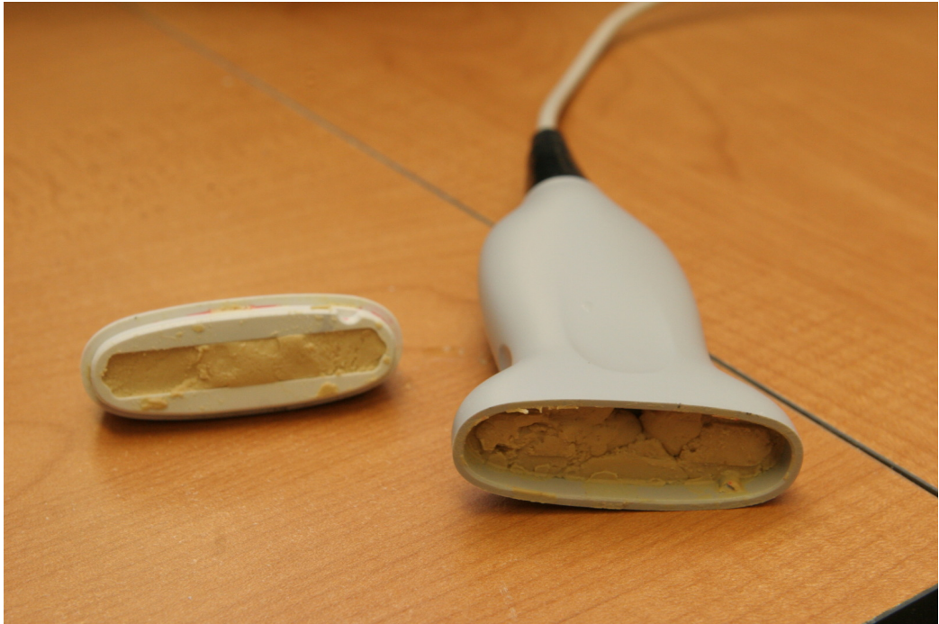
Figure 3.8: Inside of Linear Sham Transducer
