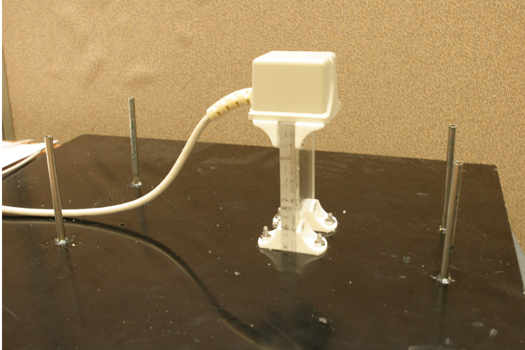
Figure 3.4: Manikin Mounting Board with Rods and Transmitter Strut
