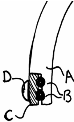
Figure 54: Sketch of Humeral Rail and Parallel Rod Mounting Method
