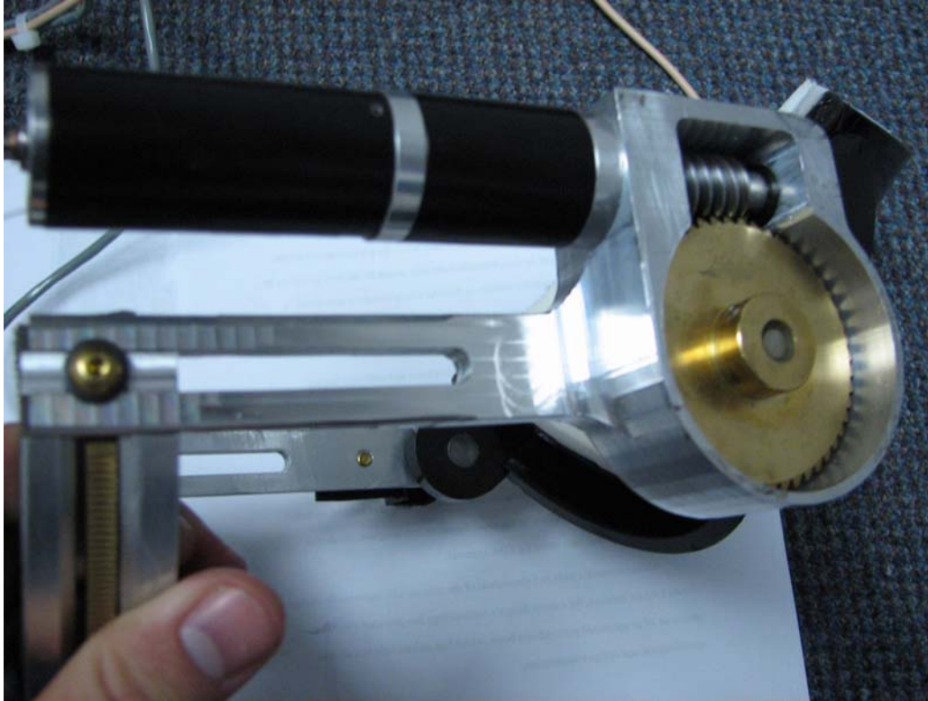
Figure 87: Fabricated Aluminum Housing
