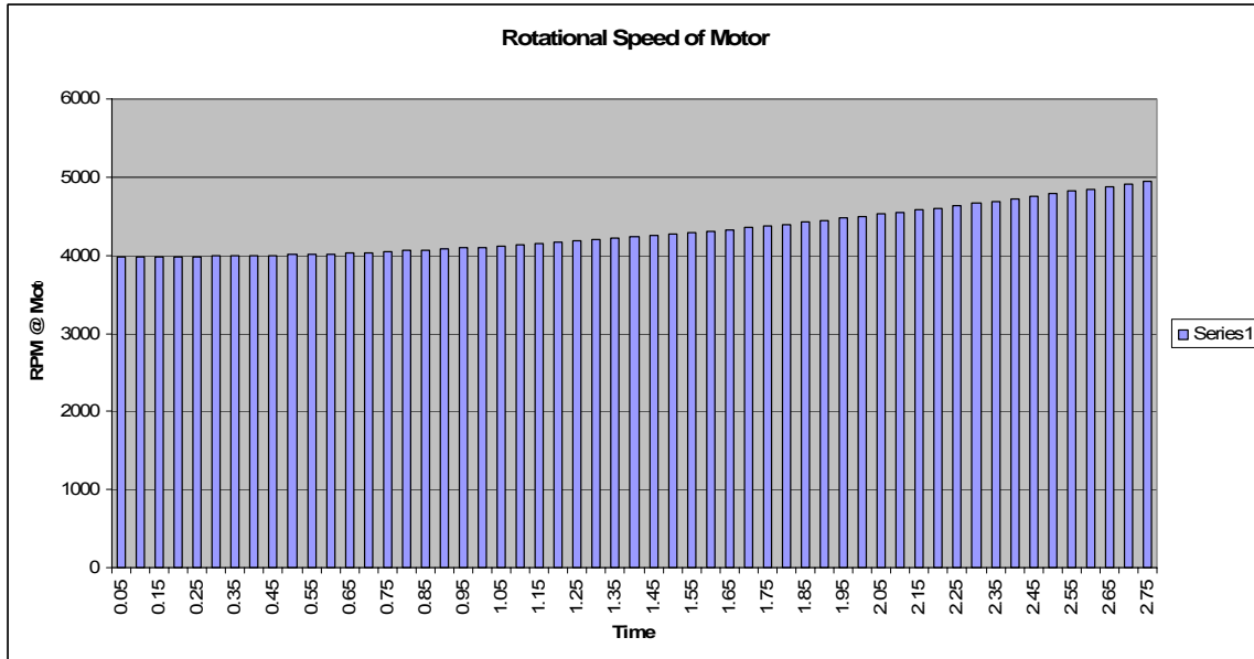
Figure 81: Humeral Motor Maximum RPM Curve
