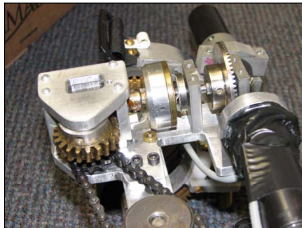
Figure 35: Proof-of-Concept Prototype Elbow Drive
