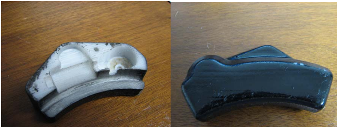
Figure 85: SLA Humeral Housing
