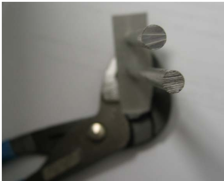
Figure 56: Twisting of Circular Rod Mate Prototype
