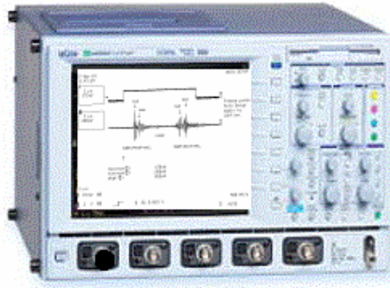
Figure 4.12 Oscilloscope (LeCroy Waverunner). Used to monitor gate location.
